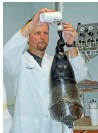
Adding catalyst-pigment mixture to activate socket lamination.
